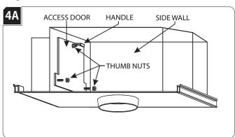
Remove the three thumb nuts and remove the access door by pulling on its handle; temporarily place it on the side wall.
