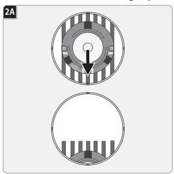
Slide the lamp housing completely out of the aperture to gain access to the transformer access door.
