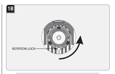
NOTE: Lamp housing can rotate 361° horizontally.
