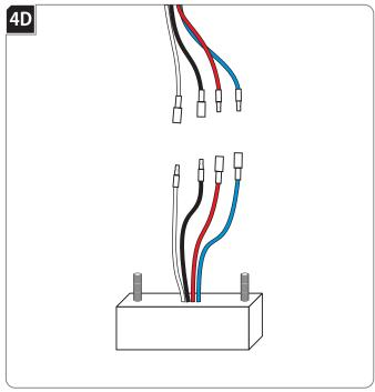
Take note of the wire connections and uninstall the old driver by disconnecting each wire connectors.
