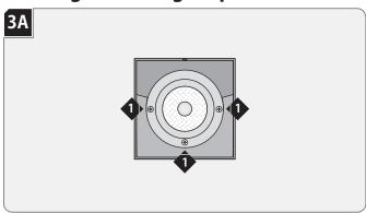
Loosen all three screws from the lamp assembly and lower the lamp assembly to gain access to the transformer access
