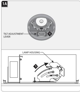
Unlock the tilt adjustment lever by pressing where indicated using a finger or screwdriver and position the lamp housing until it is completely tilted open.
