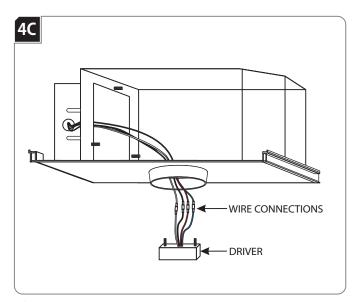
3 Slowly pull the wires out of the housing until the driver and wire connections can be accessed below the ceiling.
